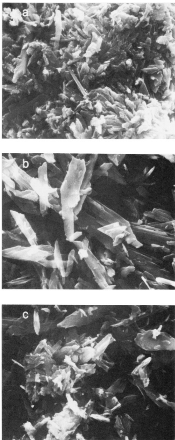
Figure 3. SEM micrographs of various UFSq samples: (a) as-synthesized, (b) from \text{CHCl}_3 extraction, (c) from \text{CH}_2\text{Cl}_2 extraction.
